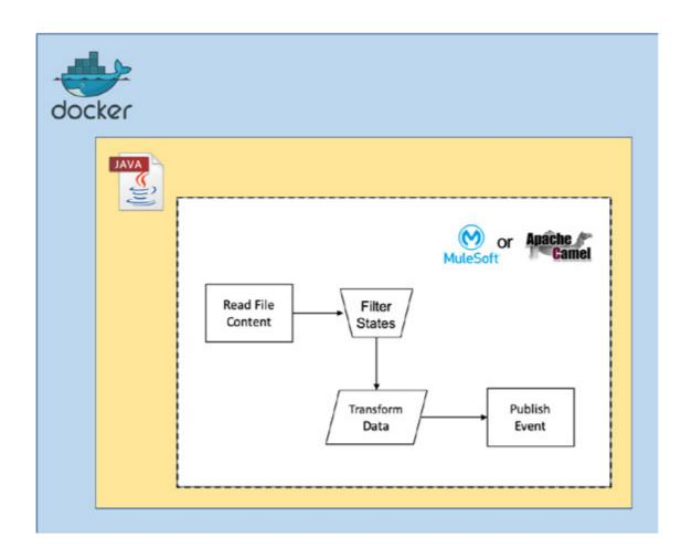
This image shows a blueprint of the anatomy of a Microflow. The integration flow is implemented in an Integration Framework Library like Mule or Apache Camel, wrapped in a JAR file, and hosted in a Docker Java image.
