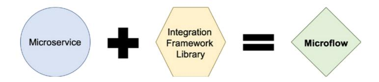
The main reason for using an Integration Framework Library like Mule or Apache Camel is to take advantage of the implemented 65 integration patterns [3]. The implementation of the patterns is proven, tested, and maintained in these integration libraries, so we do not need to reinvent the wheel and custom implement them when we want to use a Microservices approach instead of an ESB.
